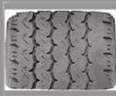
Rapid Shoulder Wear
