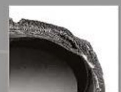
Shoulder Separation – A groove worn in the shoulder of the tire, is usually evidence of separation
