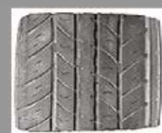
Shoulder Separation – A groove worn in the shoulder of the tire, is usually evidence of separation
