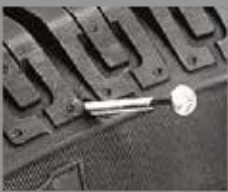
Puncture – Normally, the only evident of a puncture will be a cut that extends from the tread of the tire through the inner liner.
